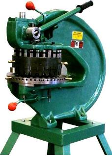
Introducing the Tin Knocker No. 18 Hand Turret Punch. A fast, accurate and flexible method of punching in the shop. Change punch & die sizes in seconds, not minutes. Priced at what you would expect to pay for a used ROTEX style machine, these 18 stations, 8-ton punch is built to last. The solid cast and machined C frame and precision machined, and ground turret make for smooth effortless punching over the user's lifetime. Accepts ROTEX punches and dies.
